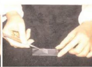
3. Lower the cover glass slowly to avoid air pockets, pull the tweezers out.
