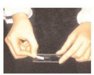
4. After placing the cover glass, the excess water should be absorbed with paper.
