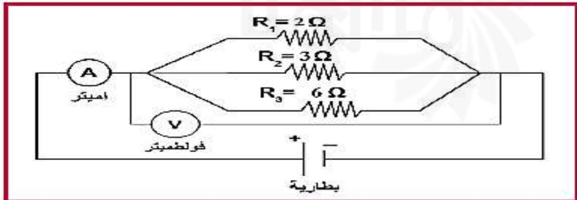
$$\frac{1}{R_{eq}} = \frac{1}{R_1} + \frac{1}{R_2} + \frac{1}{R_3}$$
